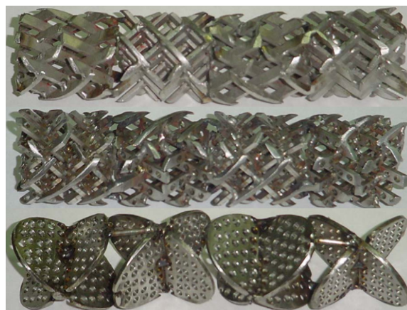
Fig. 1. Geometry of 4-element Sulzer SMX, YHC and YNU elements.
